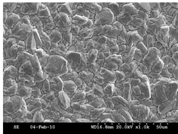
FIG 11. SEM PHOTOMICROGRAPG OF COPPER DEPOSITS OBTAINED FROM COPPER SULPHATE BATH
