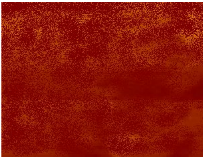
Figure 4 - AFM image of aluminum oxide on silicon dioxide film which has been grown on Si(111) substrate at 500 0 C, and 20 minutes oxygen and evaporated Al.
