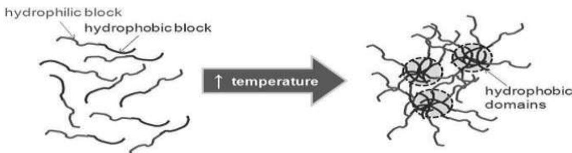
**Figure 1: Mechanism of Temperature triggered *in-situ* gel.**
