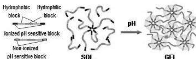
**Figure 2: Mechanism of pH triggered *in situ* gel system.**
