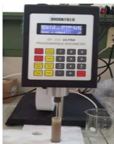
Figure 1:Viscosity measurement using a Brookfield RV DVIII rotating viscometer
