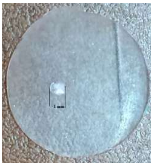
Fig. 3. The Laser damaged crystal image of SR method grown <101> directed Neodymium doped KDP crystal
