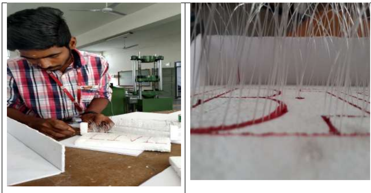
Figure 8 Inserting of Optical Fibre
