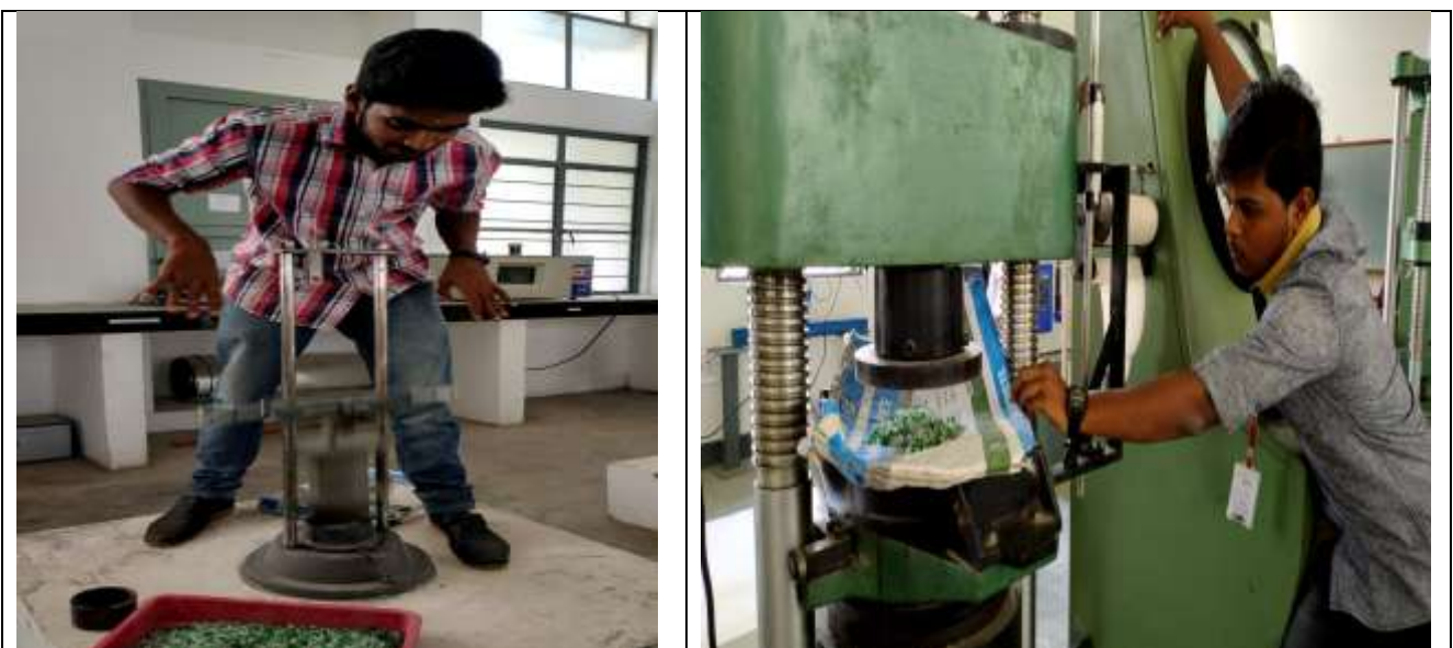
Figure 6 Preparing of glass fine aggregate
