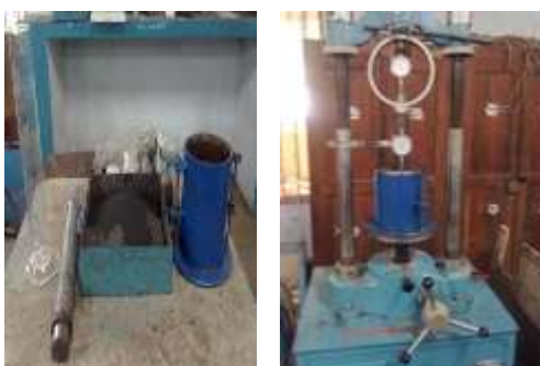
Figure.8 CBR Test with compacted sample
