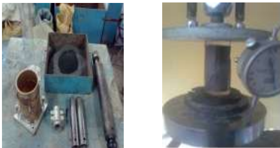
Figure.4 UCC test apparatus with specimen
