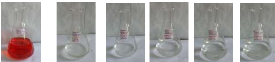
Figure -3 Congo Red Dye Solution After Standing with Quicklime Powder
