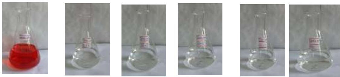
Figure -4 Congo Red Dye Solution After Shaking with Quicklime Powder
