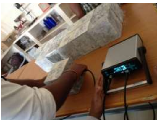
Fig.3.2 Ultrasonic Pulse Velocity test of cubes
