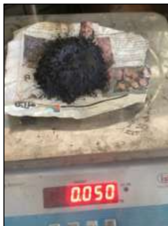
Figure.2 450 gms of aluminium with 50 gms of SiC
