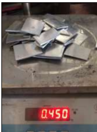
Figure.2 450 gms of aluminium with 50 gms of SiC
