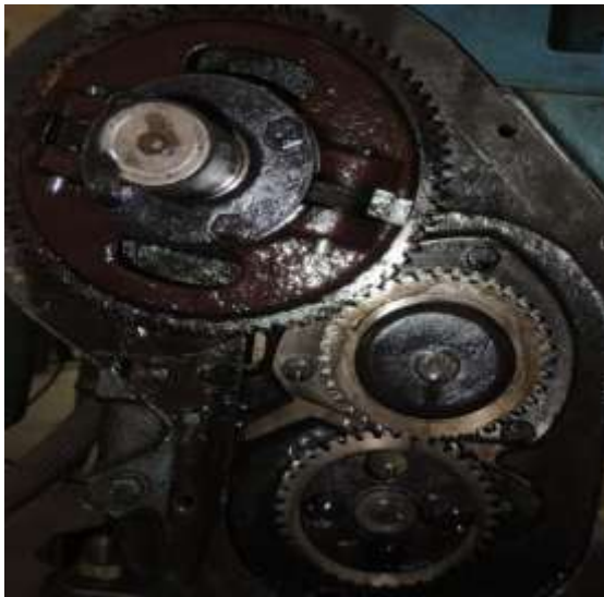
Figure 5 Varying injection timings with shim concept
