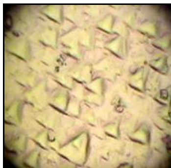
(b) Etch Pits for 5 s Average Width 5.75 \mu\text{m}
