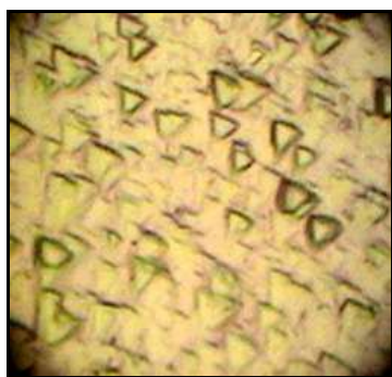
(a) Etch Pits for 2 s Average Width 2.85 \mu\text{m}
