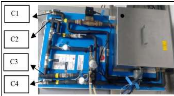
Figure 2. Unit base of the plate heat exchanger
