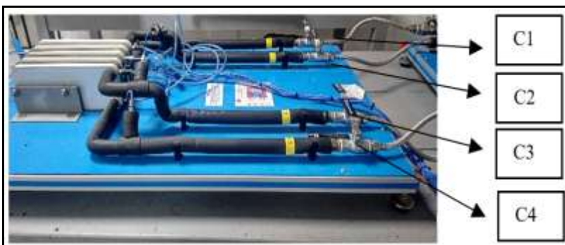
Figure 3. Extended plate heat exchanger TIPLA
