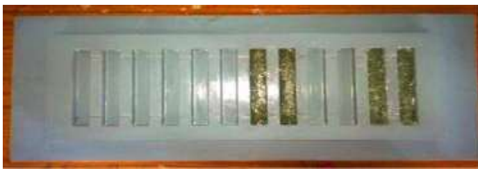
Figure 2 Wooden Die for Lay up the Laminates
