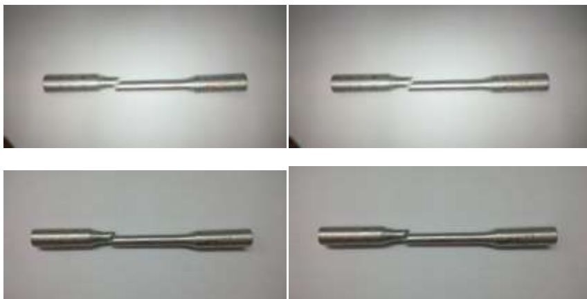
Figure 5. The photos show fracture shape experienced Specimens.
