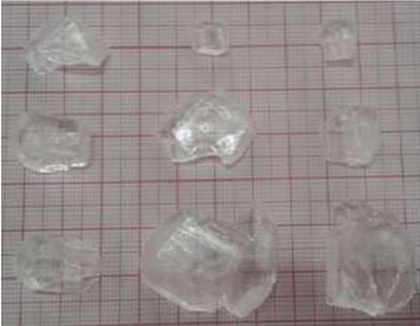
Figure 3. Photograph of TGS:ADP(8:2)single crystals
