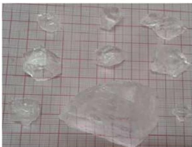
**Figure 2. Photograph of TGS:ADP(9:1) single crystals**
