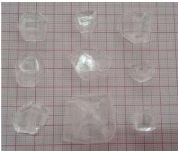
**Figure 1. Photograph of Pure TGS single crystals**
