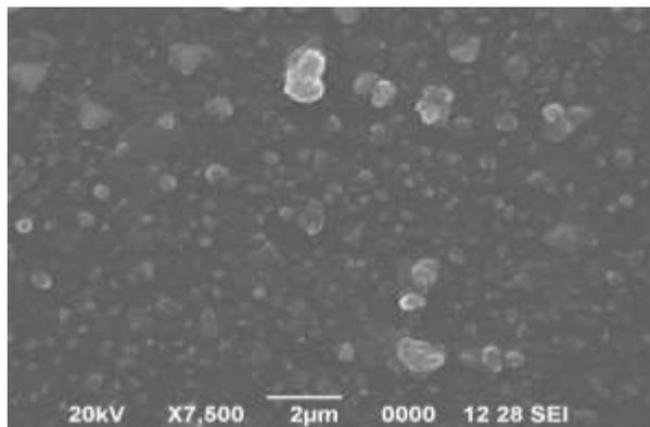
Fig .2 SEM micrograph of (c) PbS-CdS-PVA
