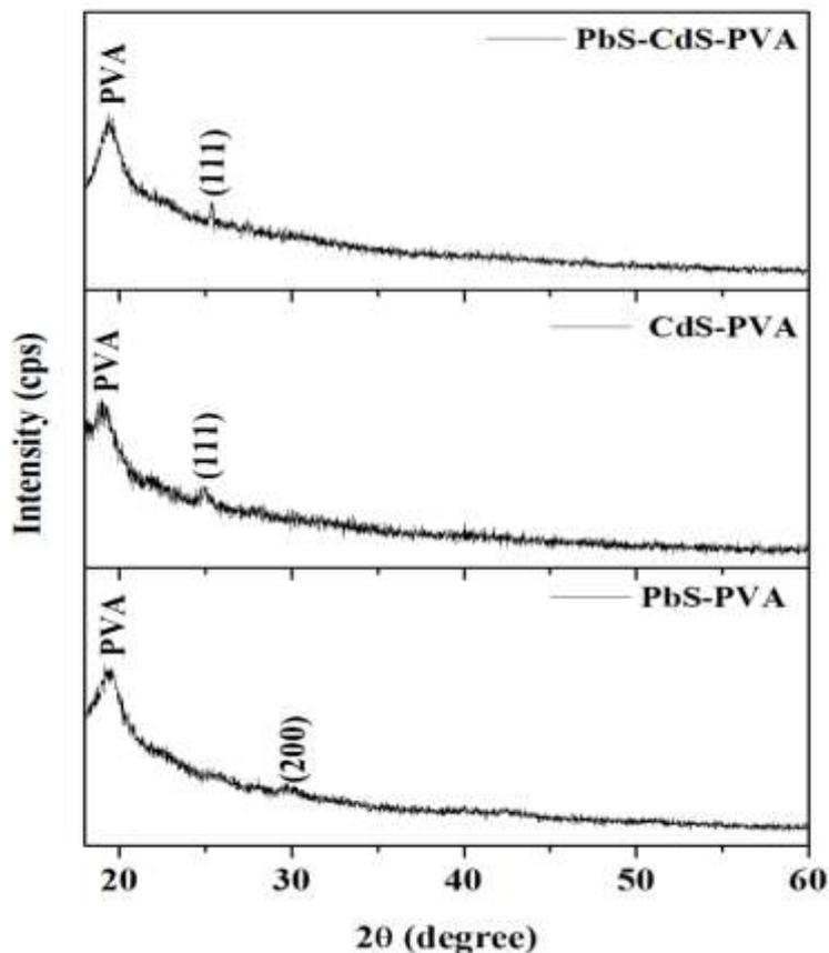
Fig. 3.1 XRD pattern of PbS-PVA and CdS-PVA and PbS-CdS-PVA nanocomposite films
