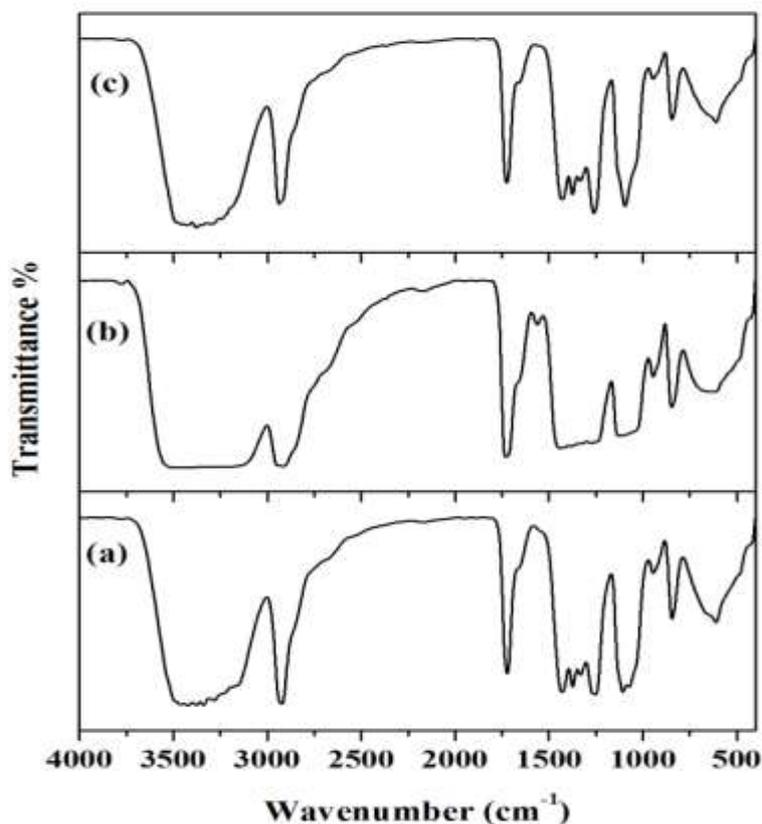
Fig.3.3 FTIR spectra of (a) PbS-PVA, (b) CdS-PVA and (c) PbS-CdS PVA nanocomposite films
