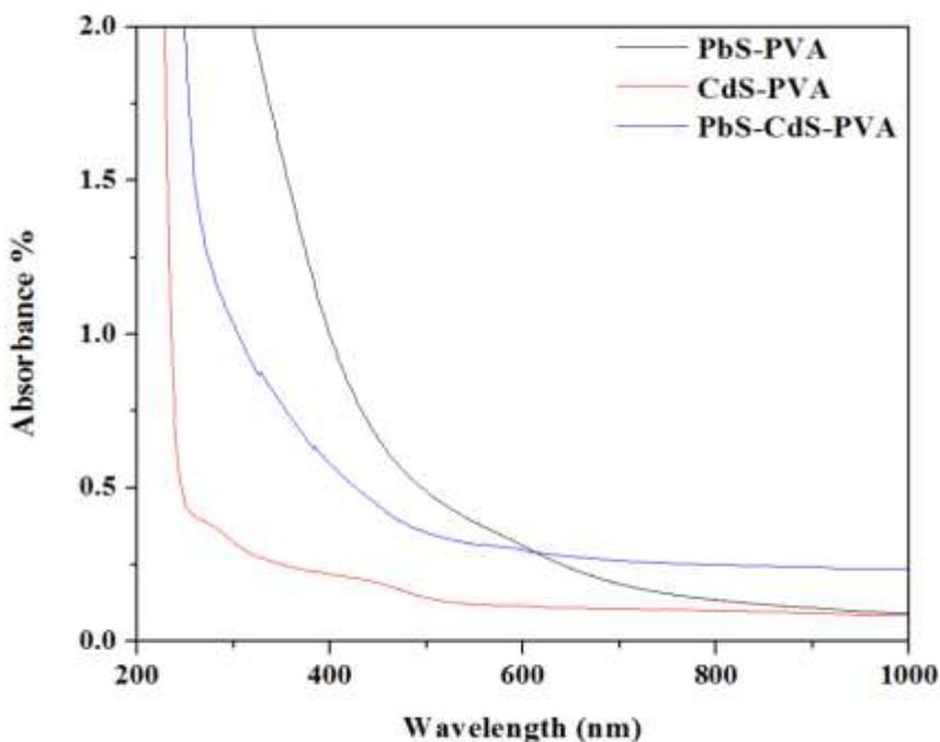
Fig. 3.4 Optical absorption spectra of PbS-PVA and CdS-PVA and PbS-CdS-PVA nanocomposite films
