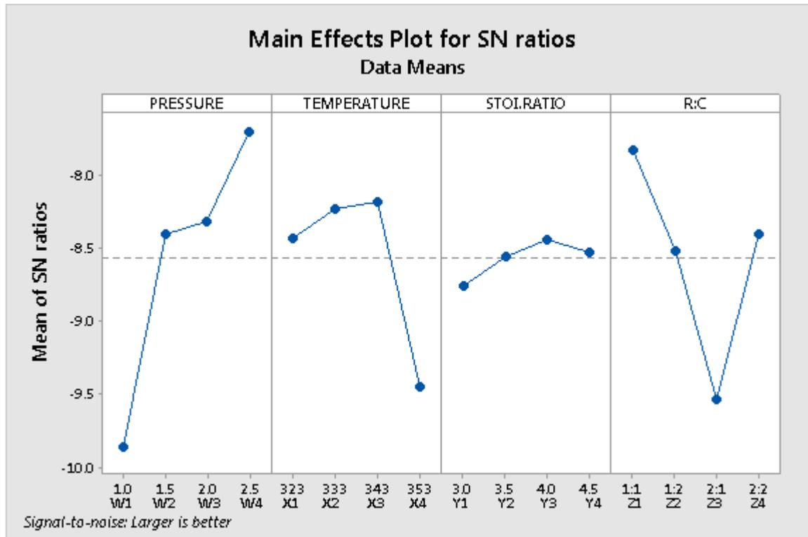
**Fig .3. Mean S/N ratio plot for R:C (W1-W4),Pressure (X1-X4),Temperature (Y1-Y4), Stoi.Ratio (Z1-Z4)**
