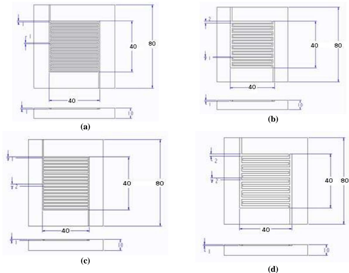
**Fig.1.Various rib to channel width (R: C) (a)1:1 (b)1:2 (c)2:1 and (d)2:2 of interdigitated flow channel of 16 cm<sup>2</sup> active area of PEM FUEL CELL**
