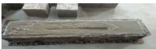
Fig 4.1 Artificial Crack Created In Conventional Concrete beam Using thin copper plate.
