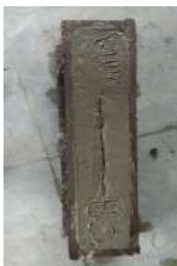
Fig 4.2 Artificial Crack Created In bacterial Concrete beam Using Thin Copper Plate
