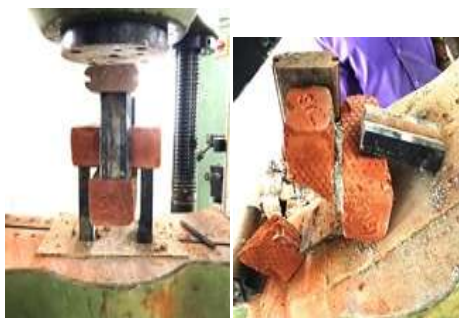
Figure 1: Test arrangement and failure mode of brick couplet
