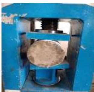
Fig 3. Split tensile test
