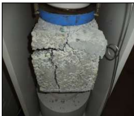
Fig. 9 – Crack pattern of Zig Zag Pattern Blocks (ZPB)
