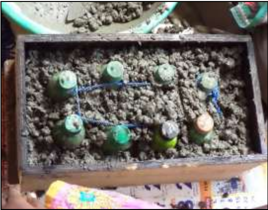
Fig. 5 – Arrangement of bottles in equal spacing pattern
