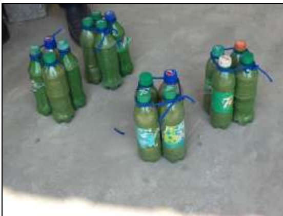
Fig. 3 – Plastic bottles filled with sand
