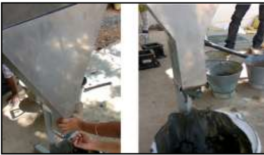
Fig. 6. Progress of V-funnel test
