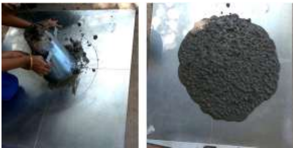
Fig. 4. Progress of slump flow test
