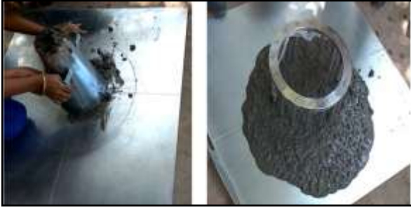
Fig. 5. Progress of J-ring test
