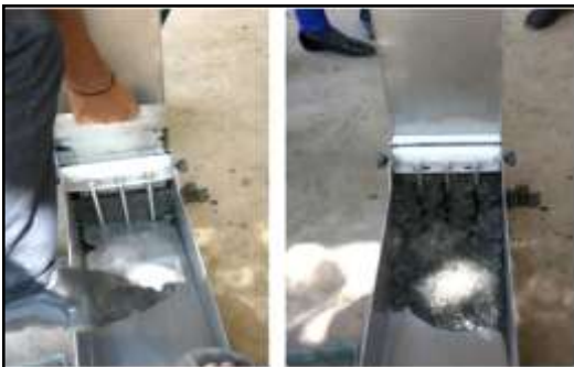
Fig. 7. Progress of L-box test
