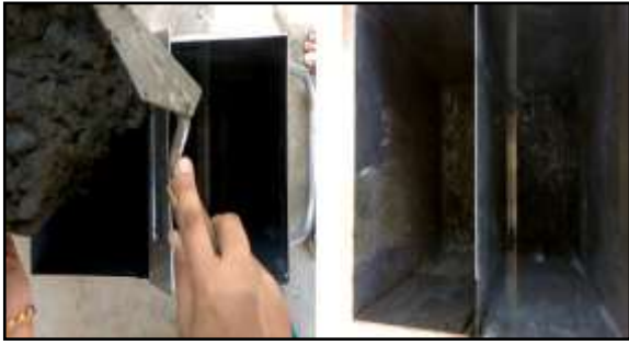
Fig. 8. Progress of U-box test
