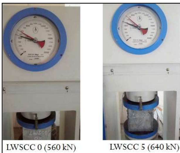
Fig. 9 Compression strength test at 7 days (LWSCC 0 & LWSCC 5)
