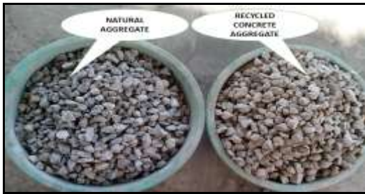
Fig 1 Natural and Recycled Concrete Aggregate
