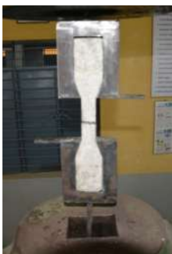
Figure.7 Typical failure of ECC under direct tensile load
