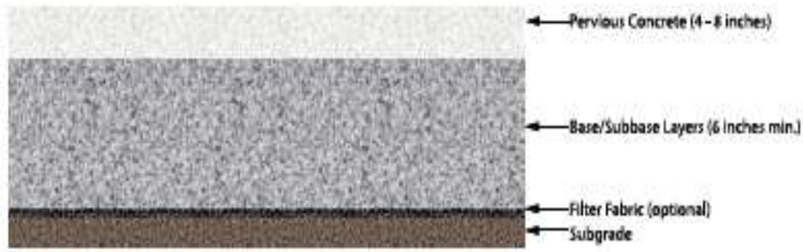
Figure 3. Typical pervious concrete pavement cross section (tech brief, FHWA-HIF-13-006)
