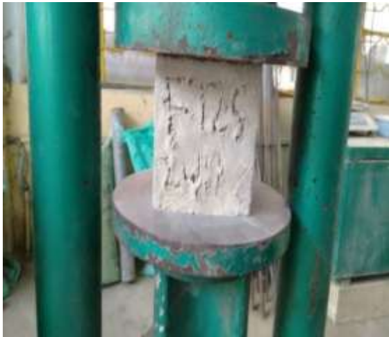
Figure 4 Cube testing for compressive strength
