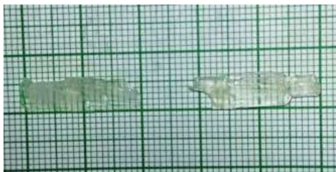
Fig. 1 Photograph of the as grown LVMgCl single crystal
