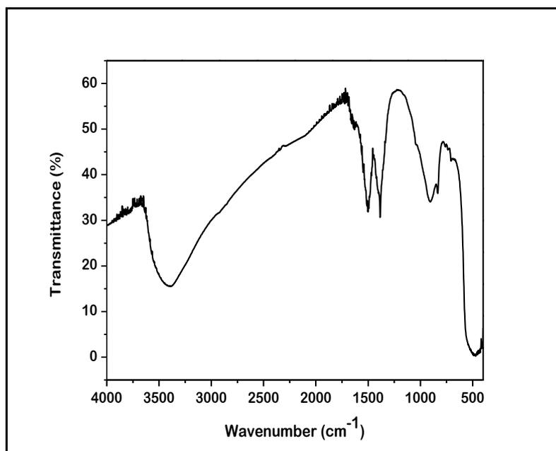
Figure 1: FTIR spectra of Zinc oxide nanoparticles
