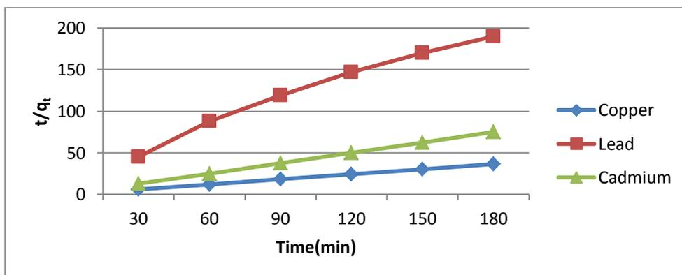
Figure 5: (b) Pseudo-second order reaction model for adsorption of heavy metals on zinc oxide doped Fenton's reagent nanoparticles
