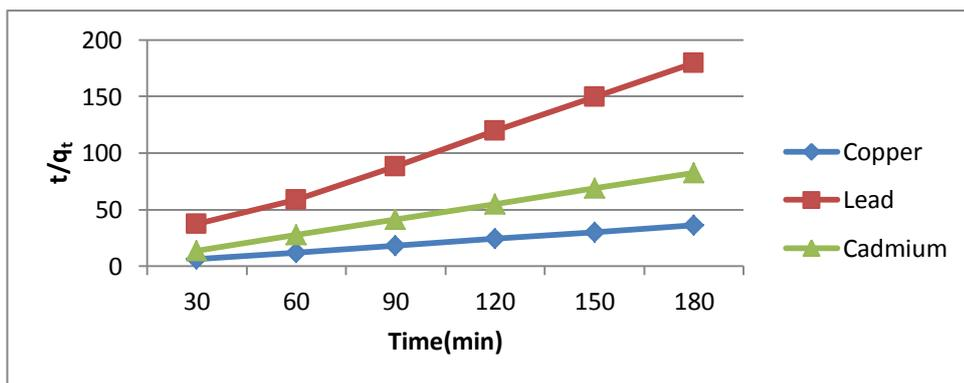
Figure 5: (a) Pseudo-second order reaction model for adsorption of heavy metals on zinc oxide nanoparticles
