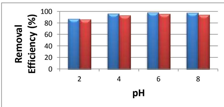
**Figure 4: (c) Effect of pH on adsorption of Cadmium (Temp = 30 °C, agitation speed = 120rpm, adsorbent dose = 0.1 g and contact time = 150 min)**
