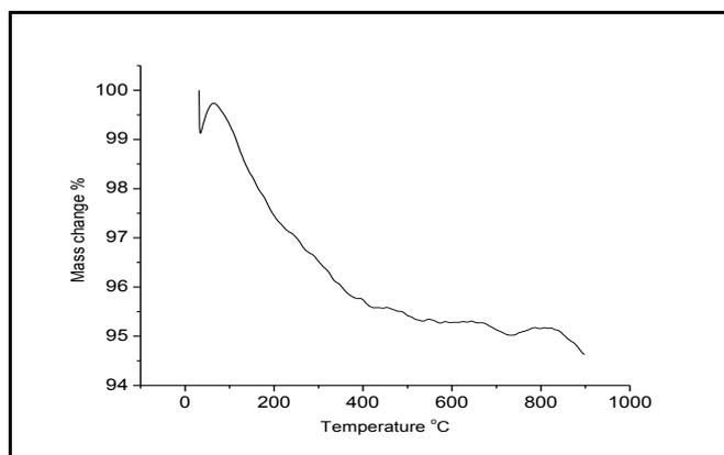
**Figure 3: TGA analysis of zinc oxide doped Fenton's nanoparticles**
