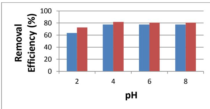
**Figure 4: (b) Effect of pH on adsorption of Lead (Temp = 30°C, agitation speed = 120rpm, adsorbent dose = 0.1 g and contact time = 150 min)**
