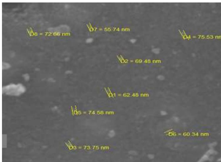
**Figure 2: SEM image of nano zinc oxide**
