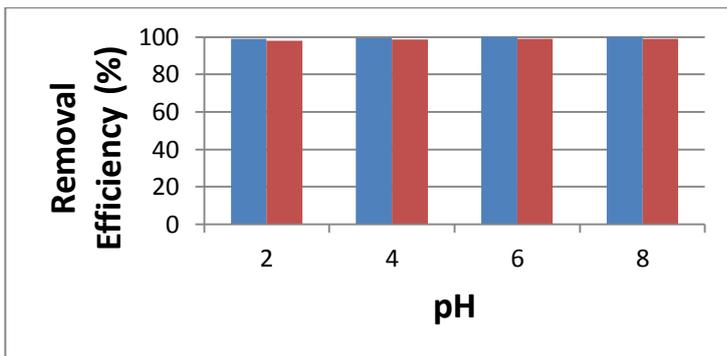
**Figure 4:(a) Effect of pH on adsorption of Copper (Temp = 30°C, agitation speed = 120rpm, adsorbent dose = 0.1 g and contact time = 150 min)**
