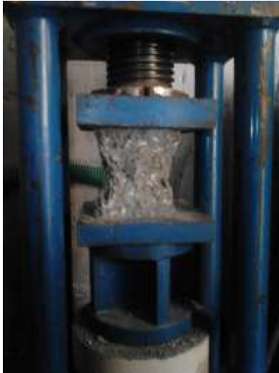
Figure 6. Compression Failure of cube
