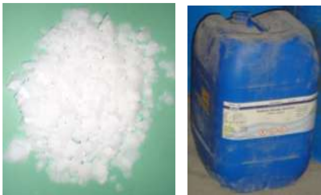
(a) Sodium hydroxide flakes (b) Sodium silicate solution Fig.1 Constituents of Alkaline solution
