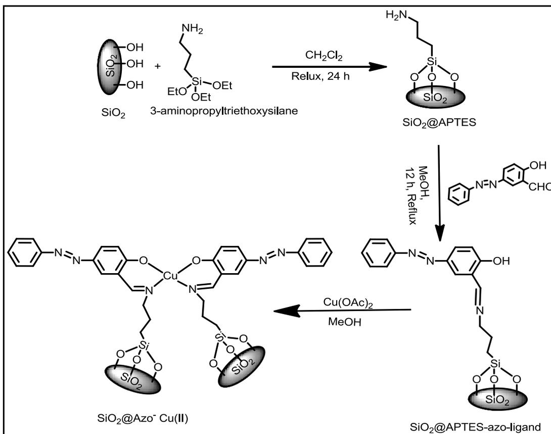
**Scheme 2. Synthesis of silica supported Azo Containing Schiff Base Copper Complex ( $\text{SiO}_2\text{@Azo- Cu(II)}$ )**
