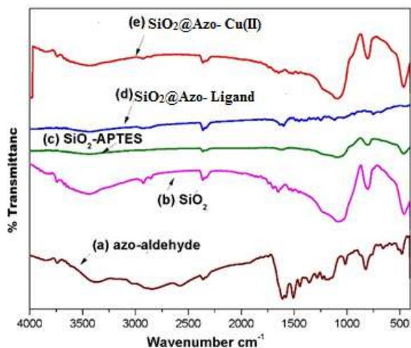
**Fig 1. FTIR-Spectra of (a) azo-aldehyde (b) SiO<sub>2</sub>, (c) SiO<sub>2</sub>-APTES, (d)SiO<sub>2</sub>@APTES-Azo-ligand (e) SiO<sub>2</sub>@Azo- Cu(II) Complex.**
