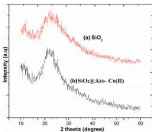
**Fig 3. X-ray diffraction patterns of patterns of (a) SiO<sub>2</sub> and (b)SiO<sub>2</sub>@Azo- Cu(II) complex**
