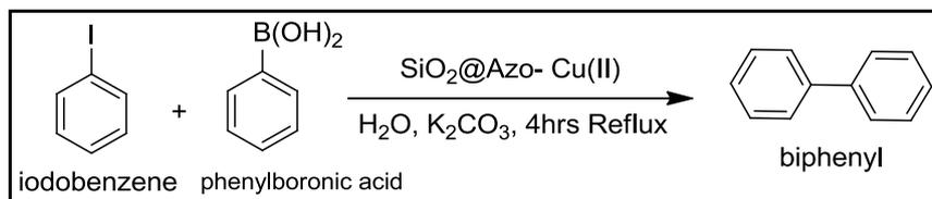
**Scheme 3.** The Suzuki–Miyaura cross coupling reactions of iodobenzene with phenylboronic acid
