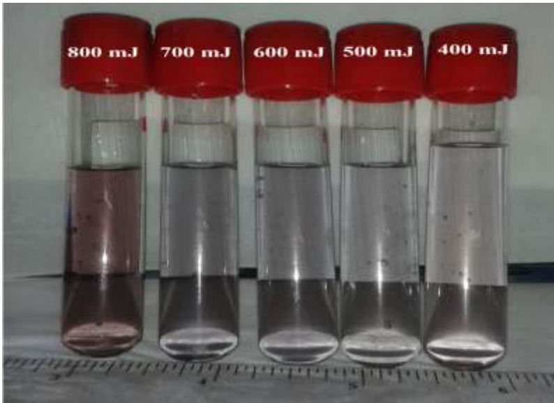
Fig (2) Water contain Au nano particles produced by laser with different power
