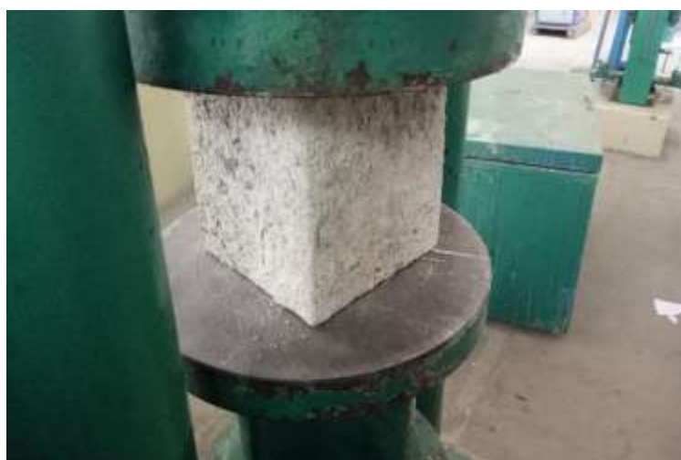
Figure 2 Cubes testing for compressive strength
