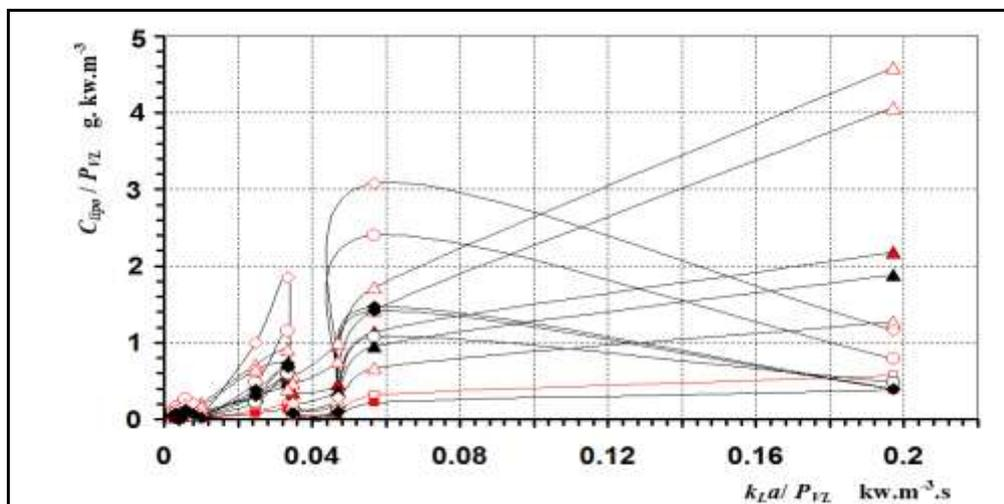
Fig. 3: Relation between  $k_La/P_{VL}$  fraction and  $C_{\text{lipe}}/P_{VL}$  ( $\Delta$  surfactins,  $\diamond$  iturins,  $\circ$  fengycins,  $\square$  kurstakins)
