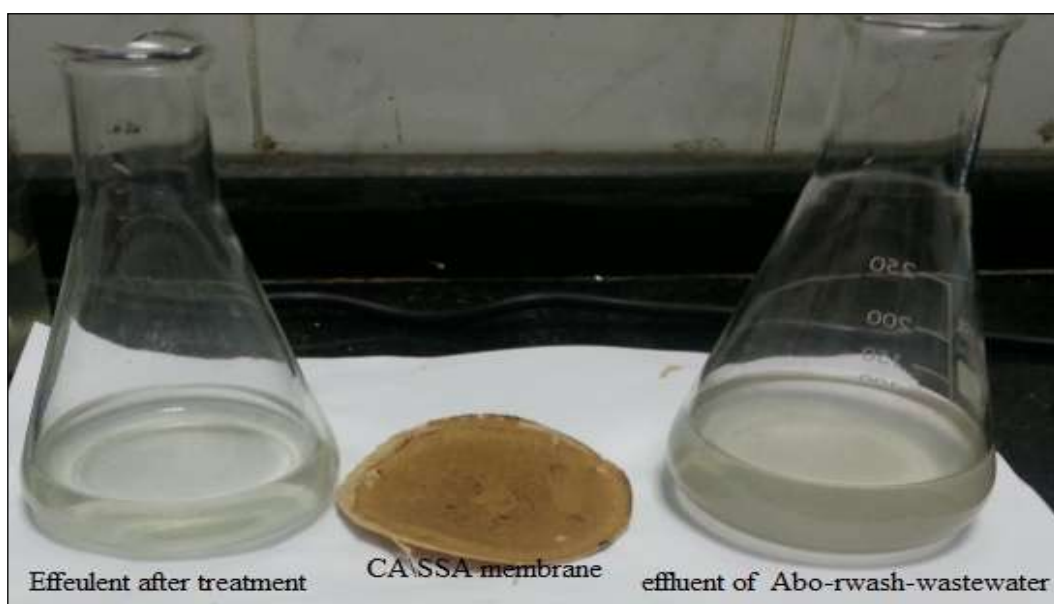
Figure (8) Images of wastewater from Abo-Rwash plant before and after treatment with CA\SSA blend membrane at 50/50 Wt%
