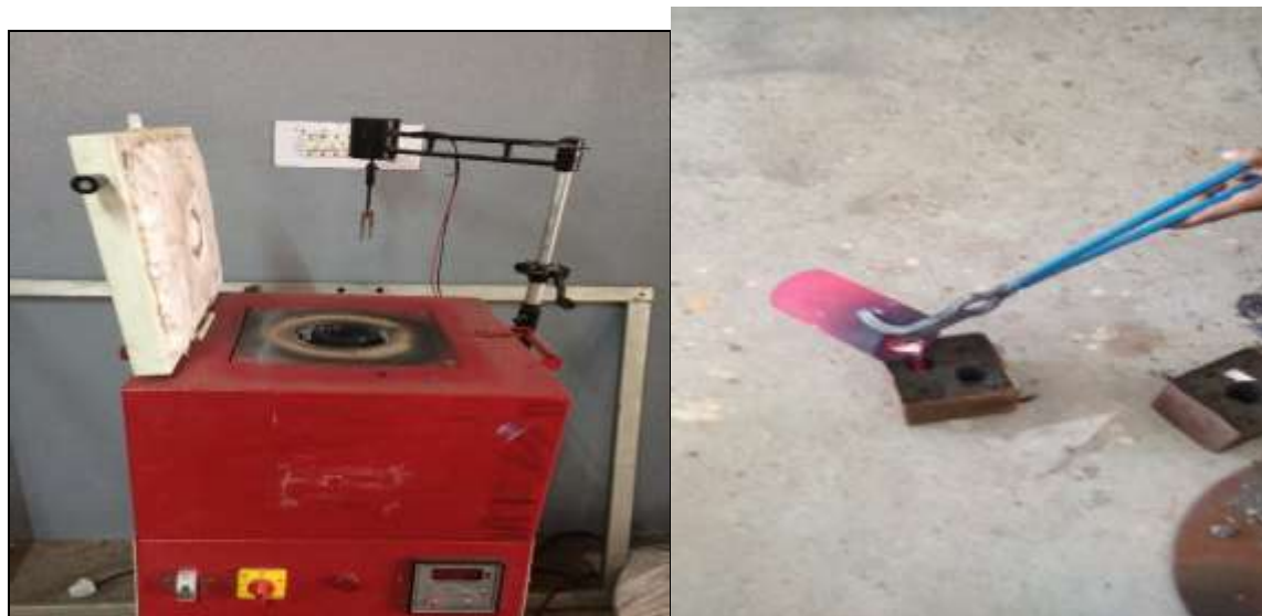
Fig 1. Stir casting equipment. Fig 2. Casting process
