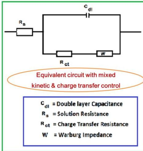
**Figure 4. Equivalent circuit diagram for AC impedance spectra**
