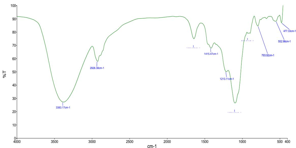
**Figure 5. FTIR spectrum of pure CVWT**
