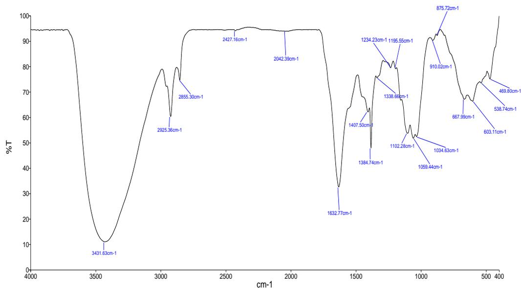
**Figure 6. FTIR Spectrum of NiTi shape memory alloy immersed in AS containing CVWT (1%)**
