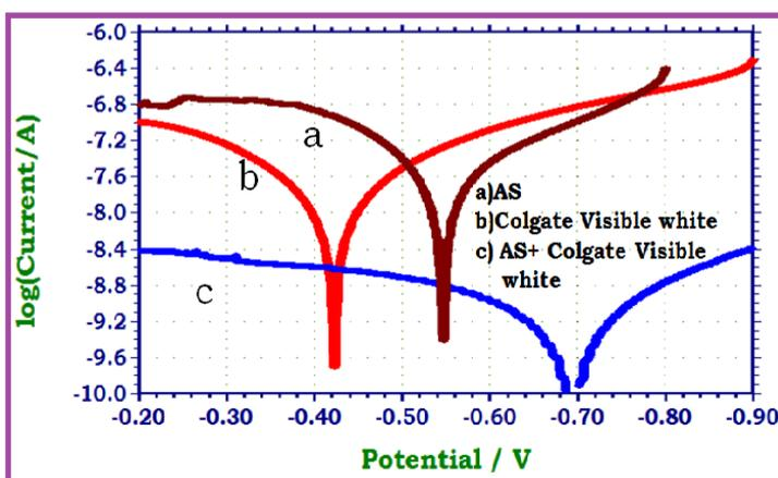
Figure 1. Polarization curves of NiTi shape memory alloy immersed in AS in the absence and presence of CVWT(1%) (Tafel plot)
