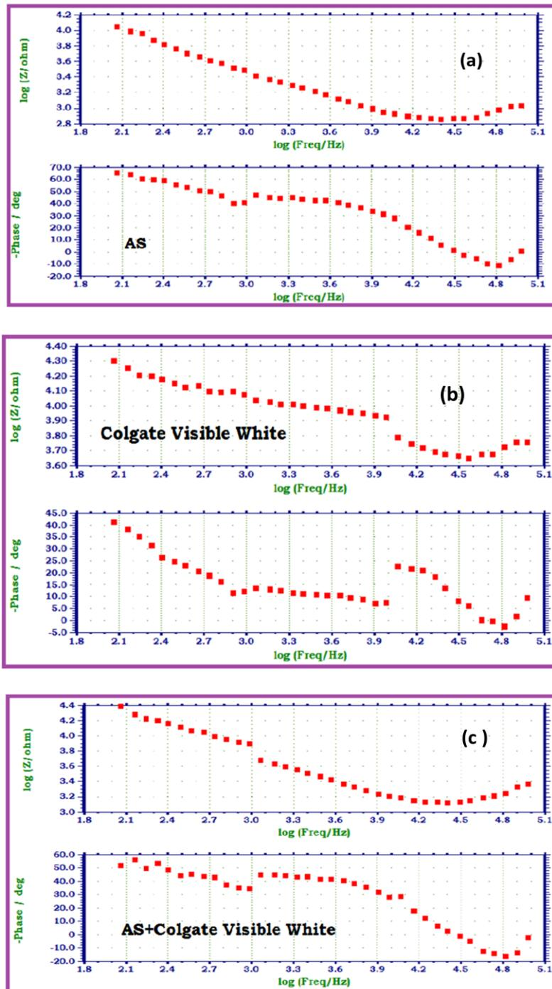
**Figure 3(a,b,c) AC impedance spectra of NiTi shape memory alloy immersed in various test solutions**
