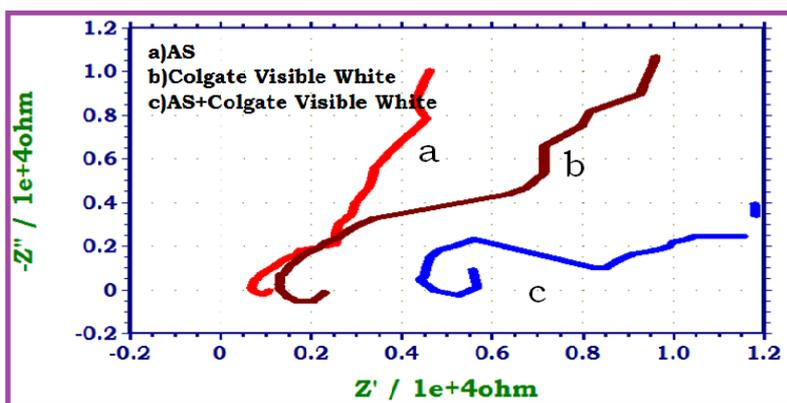
**Figure 2. AC impedance spectra of NiTi shape memory alloy immersed in AS in the absence and presence of CVWT (1%) (Nyquist Plots)**
