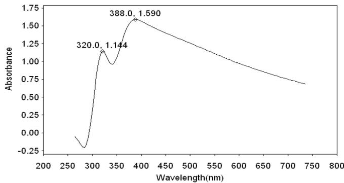
**Figure 8. UV-Visible absorption spectrum of solution containing CVWT**
