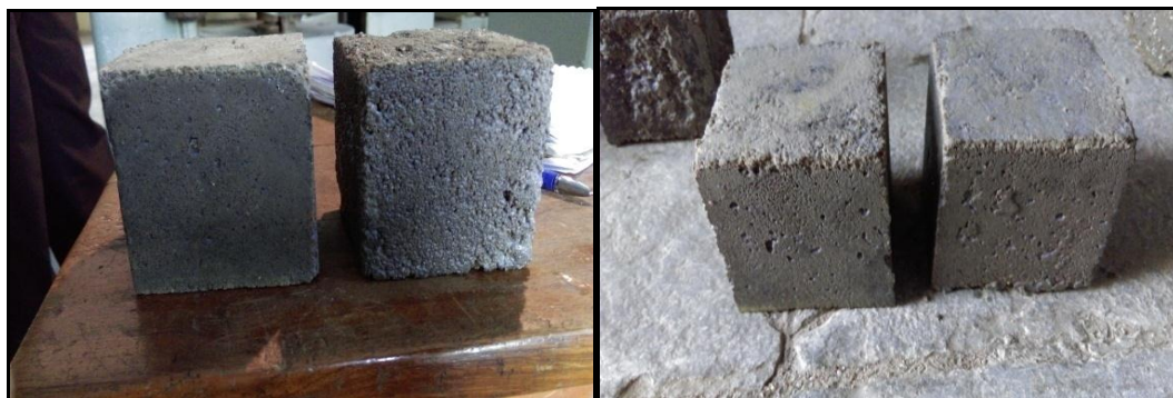
Figure 1 specimens after 90days in 5% H 2 SO 4 Figure 2 specimens after 90days in 5% HCL
