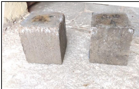
Figure 4 specimens after 90days in 5% NaCl solution.
