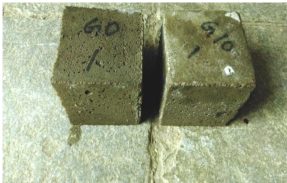
Figure 3 specimens after 90days in 5% Na 2 SO 4 solution.
