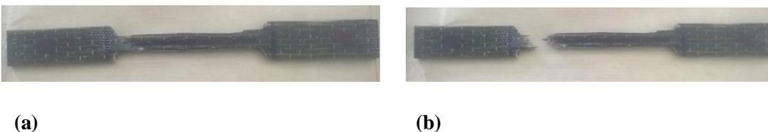
Figure 4.1 Tensile test specimens (a) before fracture and (b) after fracture
