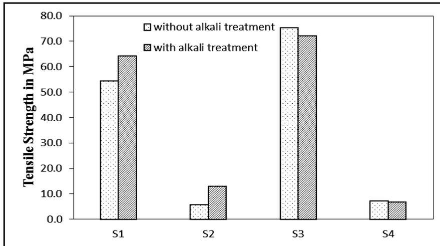
**Figure 4.2 Tensile strength comparisons of hybrid composites with and without alkali treatment**
