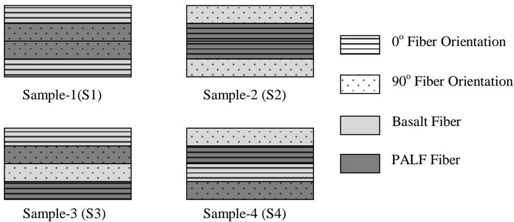
**Figure 2.4 Stacking sequence and fiber orientation of Basalt fiber+PALF hybrid composite**
