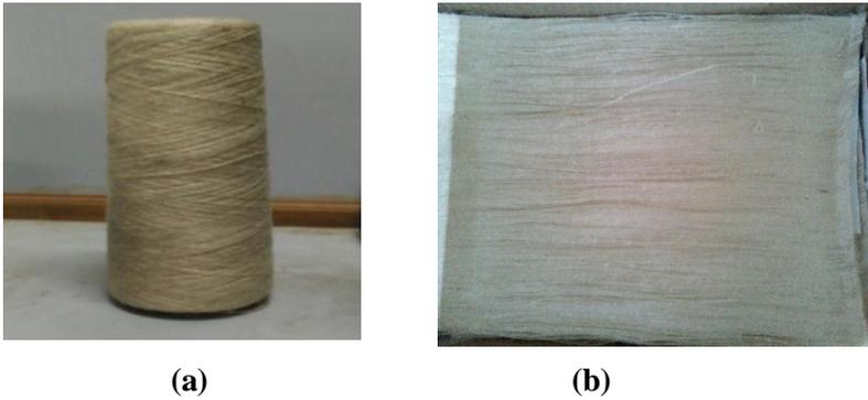
Figure 2.2 Pineapple leaf fiber (a) Continuous fiber (b) Unidirectional mat
