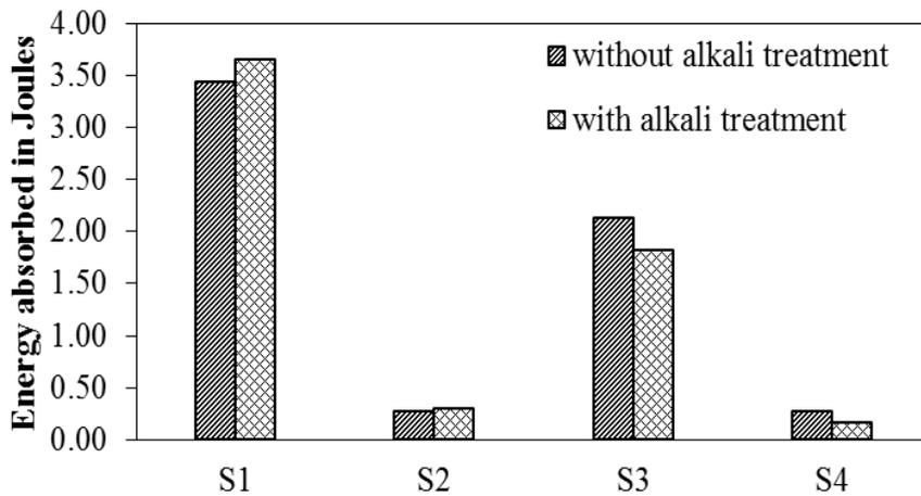
Figure 4.6 Comparisons of Energy absorption by the hybrid composites with and without alkali treatment
