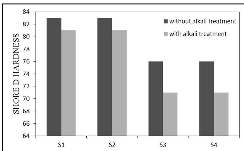
Figure 4.6 Comparisons of hardness values of hybrid composites with and without alkali treatment
