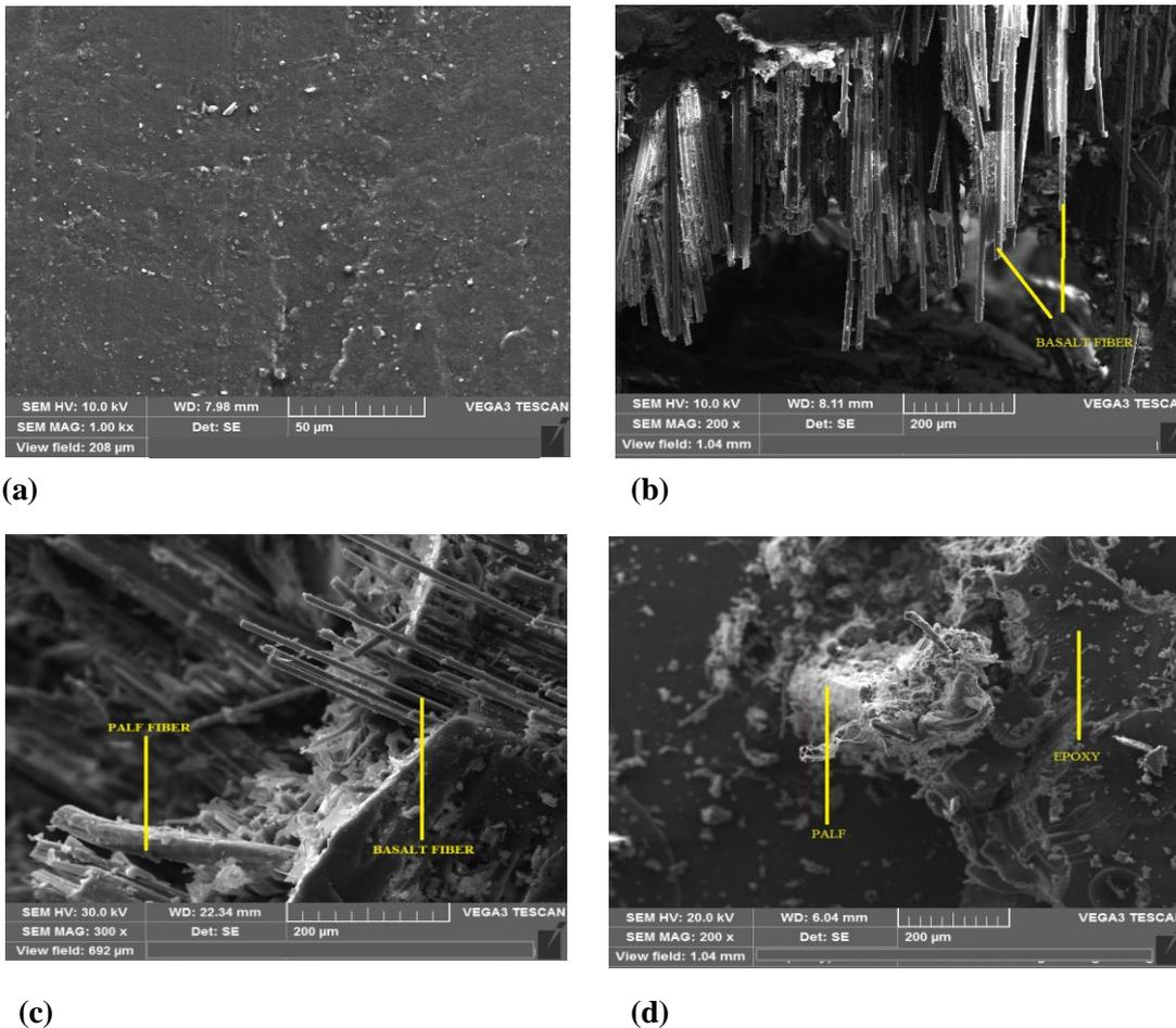
Figure 4.7 SEM image of (a) Epoxy surface (b) & (c) Tensile tested specimen (d) PALF breakage
