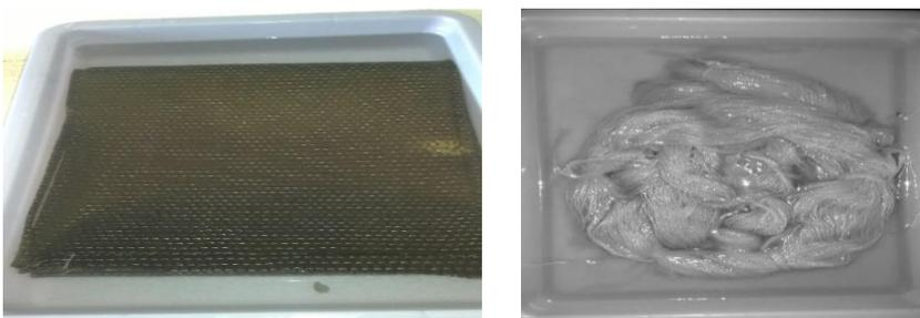
Figure 2.3 Alkali (NaOH) surface treatment of (a) Basalt fiber (b) PALF fiber
