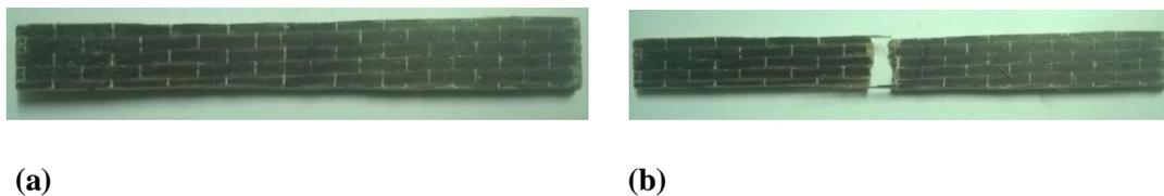
**Figure 4.3 Flexural test specimens (a) before fracture and (b) after fracture**
