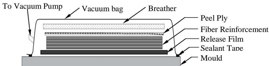
**Figure 2.5 Schematic representation of hybrid composite fabrication by Vacuum bagging method**
