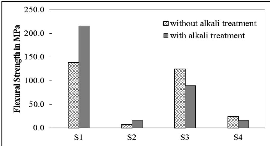
Figure 4.4 Flexural strength comparisons of hybrid composites with and without alkali treatment
