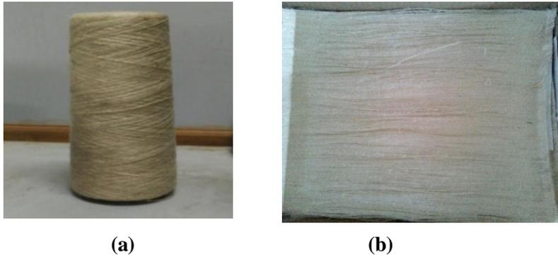
Figure 2.2 Pineapple leaf fiber (a) Continuous fiber (b) Unidirectional mat
