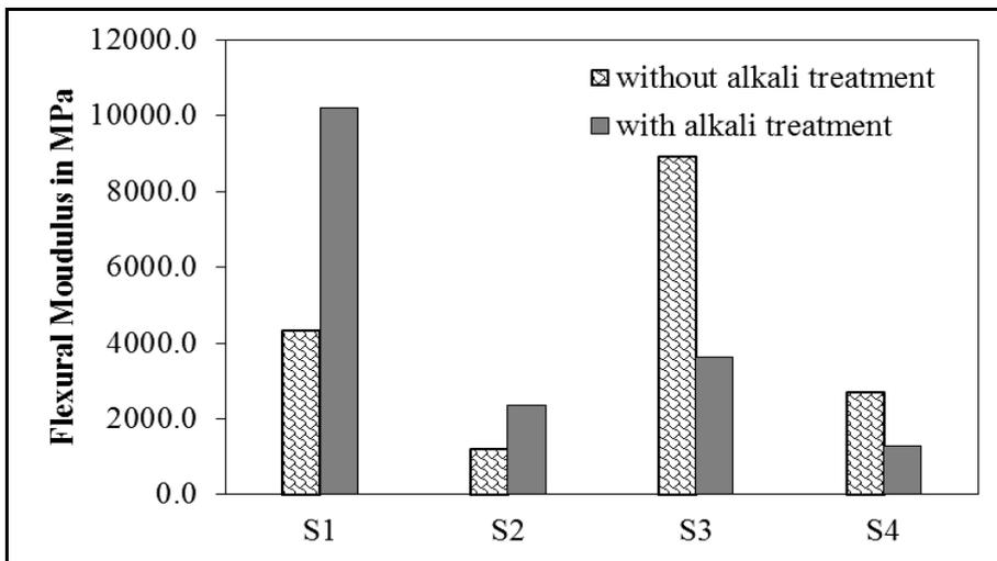
Figure 4.5 Flexural modulus comparisons of hybrid composites with and without alkali treatment
