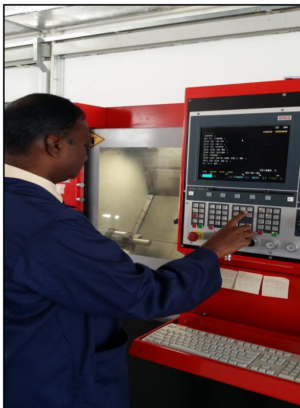
Figure 1 High speed CNC turning centre (EMCO TURN 250)
