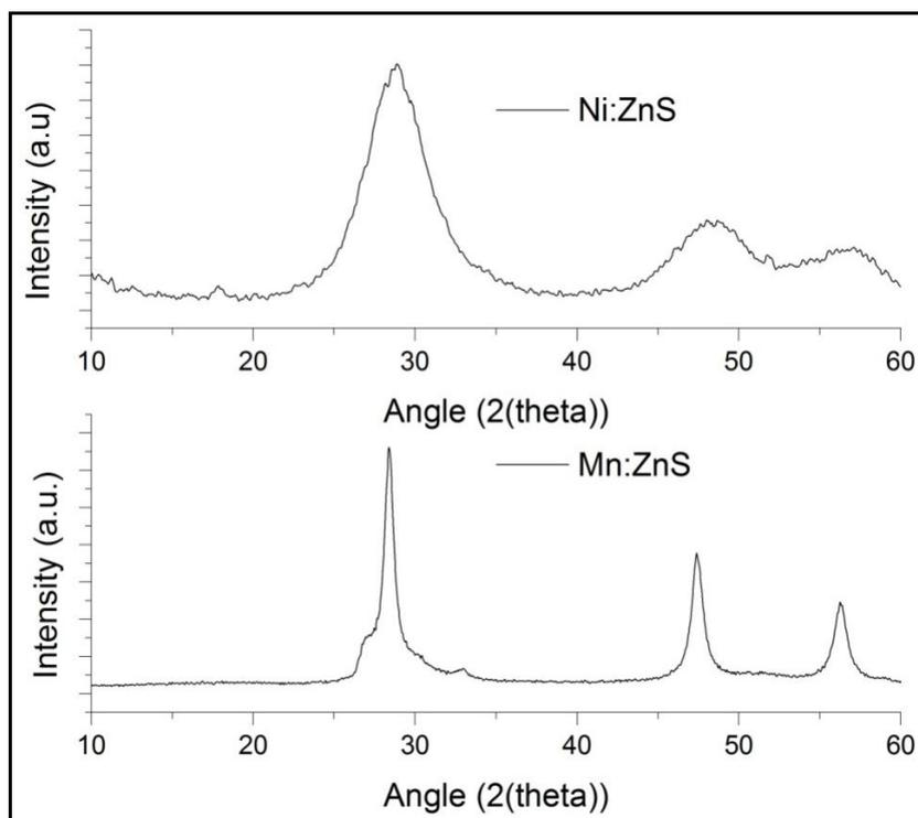
**Figure 2 XRD Pattern of Mn:ZnS and Ni:ZnS**
