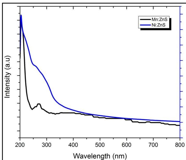
**Figure 1** UV-Visible-NIR spectra of Mn:ZnS and Ni:ZnS
