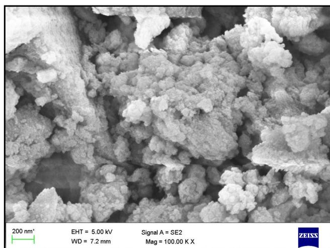
**Figure 3(b): scanning electron microgram of Ni:ZnS**
