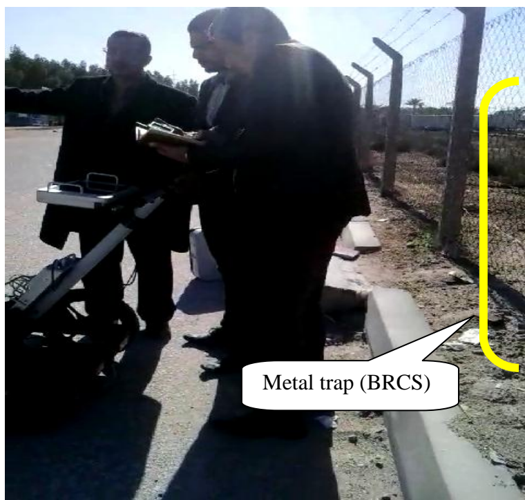
Fig. 4 Metal trap which causes abnormalities in Profile GPR No. 11
