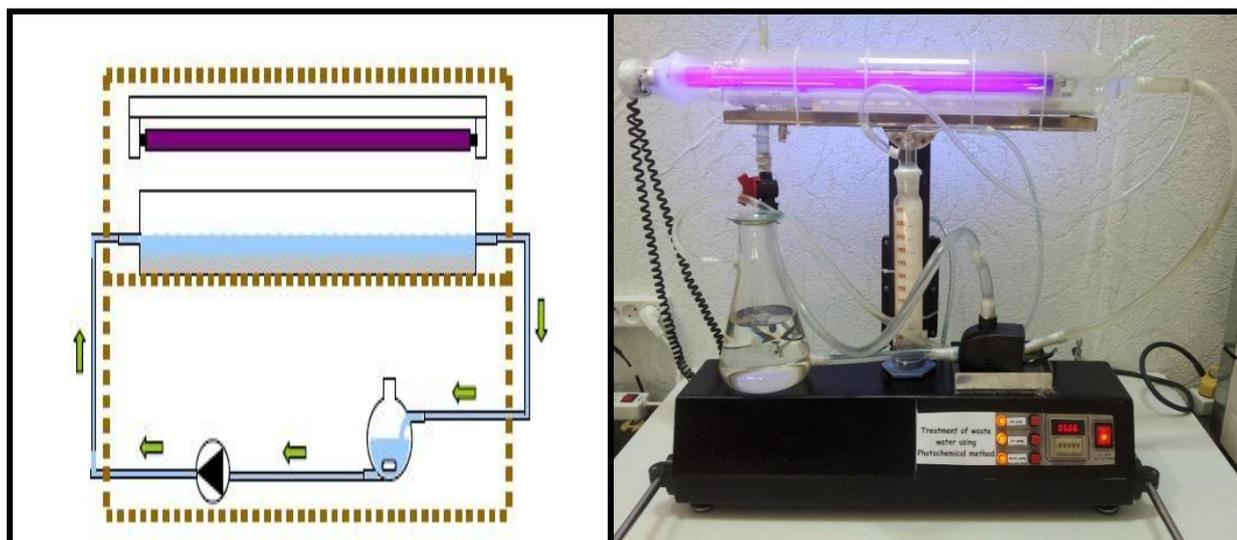
**Figure 2: The lab-scale photochemical reactor**
