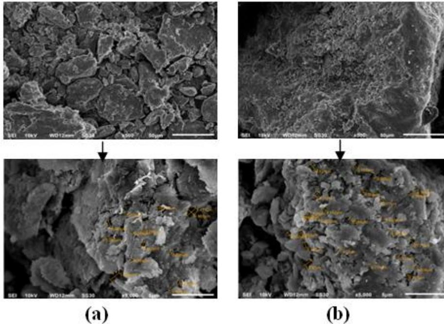
Figure1. SEM image of bentonite and ZrO<sub>2</sub>- pillared bentonite
