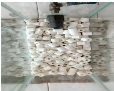
Figure 1. Ceramic media before using in reactor SBBGR
