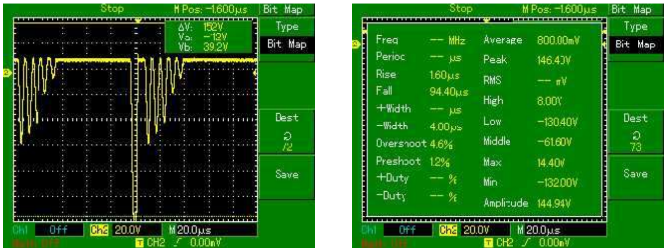
Figure 9: DSO Output Voltage with only Primary Compensated and its parameters.
