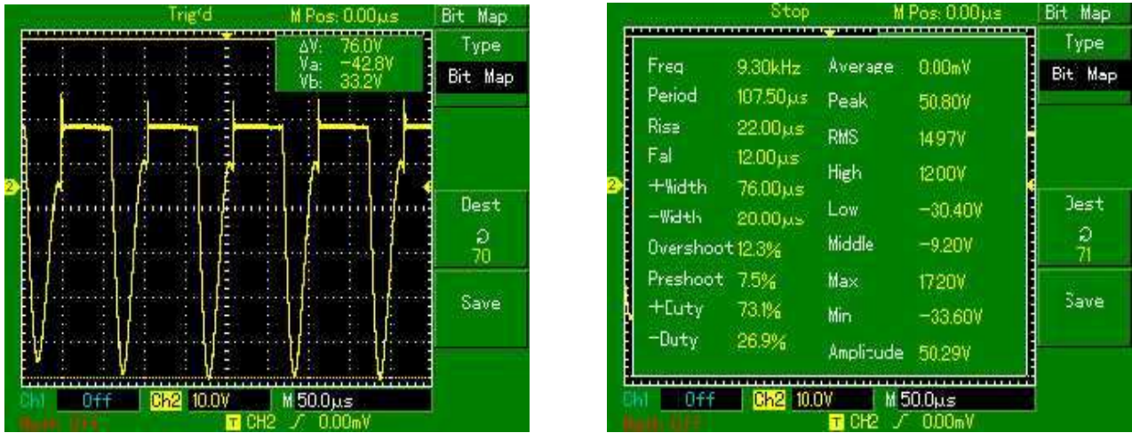
Figure 7: DSO Output Voltage of Primary with compensation and its parameters
