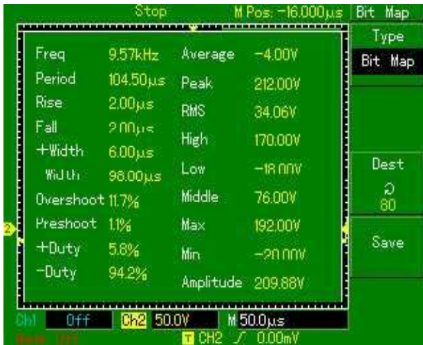
Figure 5: DSO Output Voltage of Primary coil without compensation and its parameters.
