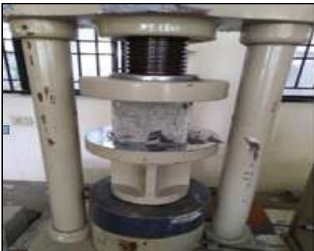
Figure 2. Compressive strength of cube
