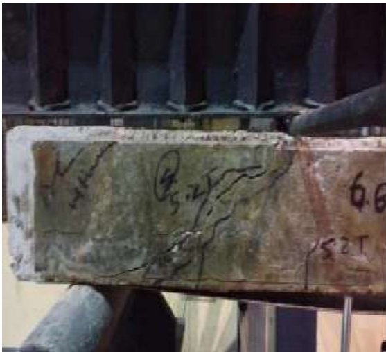
Figure 10. Failure pattern and Load-deflection curve of RC beam strengthened with 2mm thick plate
