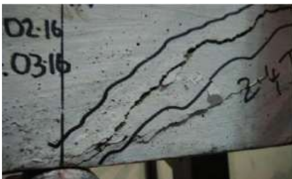
Figure 8. Failure pattern and Load-deflection curve of RC beam strengthened with 1.5 mm plate
