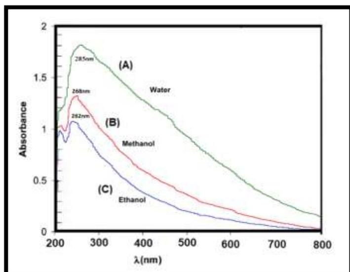
**Fig. 5: UV-Vis of CuO NPs prepared using water as solvents (A), methanol (B), ethanol (C)**
