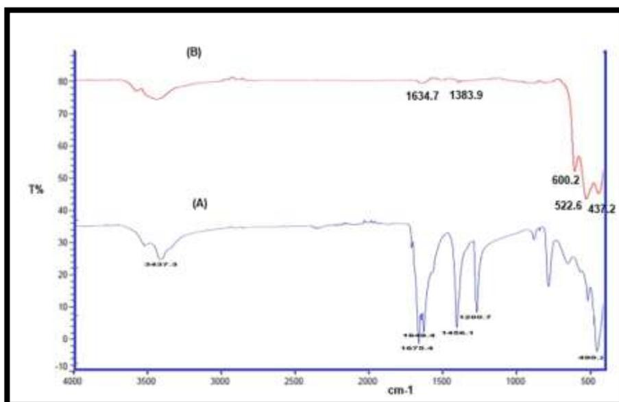
**Fig. 4:** FTIR spectrum of copper oxalate complex (A) and copper oxide NPs (B)
