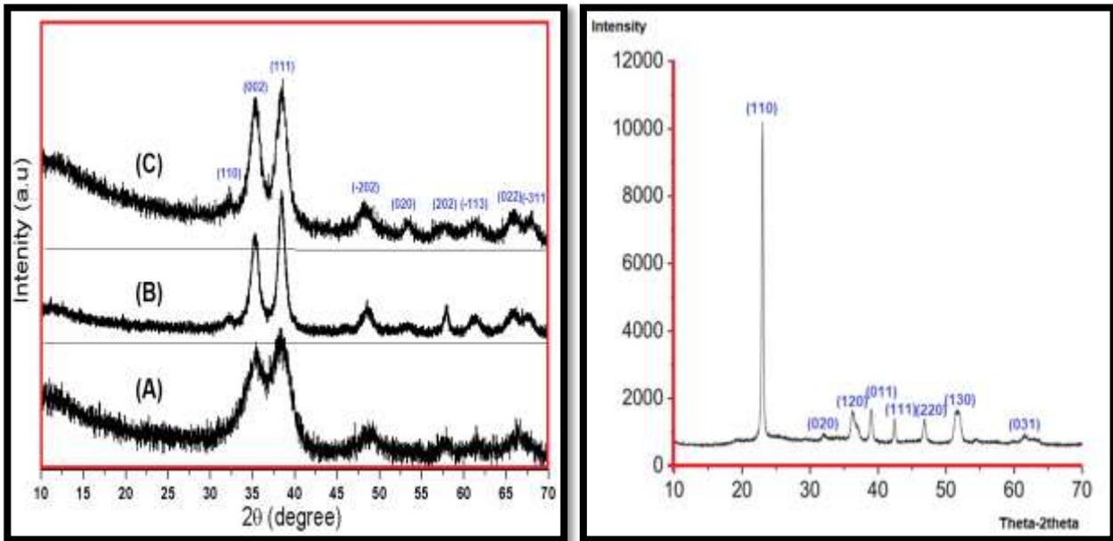
**Fig. 2:** XRD spectrum of CuO NPs prepared using ethanol as solvents (A), methanol (B), water (C) and spectrum of copper oxalate (D)
