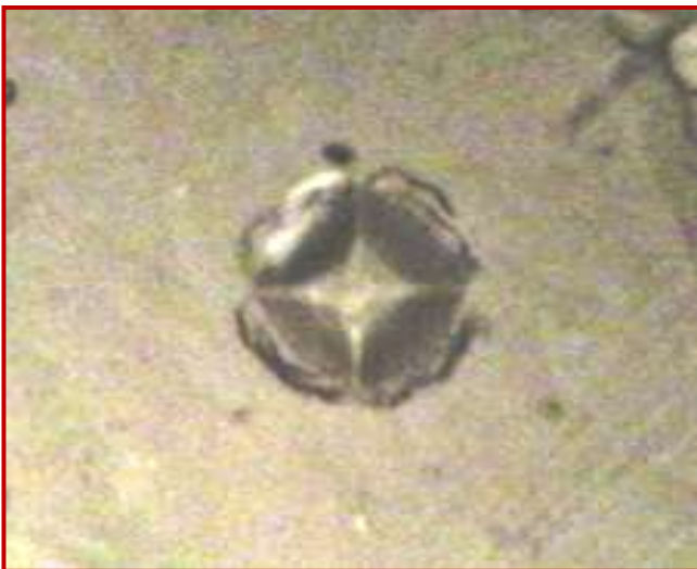
Fig.1.3 Vickers indentation image 15% of B 2 O 3 content
